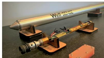
The Active-FLI probe contains internal sensors plus fibre-optic line. Data is captured by a small surface recorder box.
