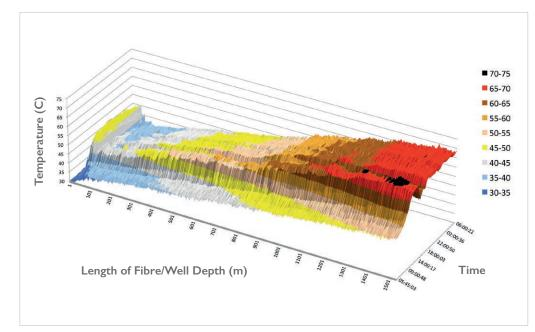
This example shows a static visualization of a time elapsed DTS log.The entire history of the cement curing process is displayed for interpretation of heating and cooling along the wellbore over time. DTS data can also be easily reproduced in video format to replay and revisit the cement cure process and behaviour.
